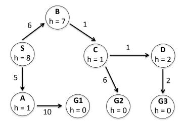
Execute weighted A<sup>\*</sup> on the above graph with  $\varepsilon = 2$ , completing the following table. To save time, you can optionally just write the nodes added to the fringe, with their g and f values.
